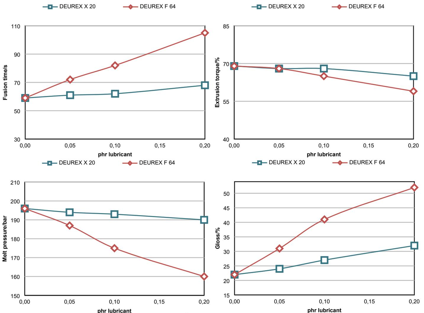
Fig. 1 to Fig. 4 Influence of the dosage of DEUREX® X 20 K in comparison to F 64 on fusion time (Fig. 1), extrusion torque (Fig. 2), melt pressure (Fig. 3) and gloss (Fig. 4)
